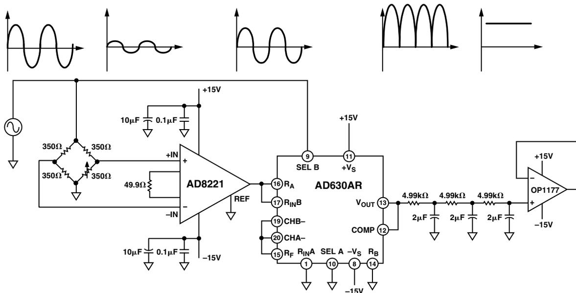
Figure 1. Using an AC Signal to Excite the Bridge
